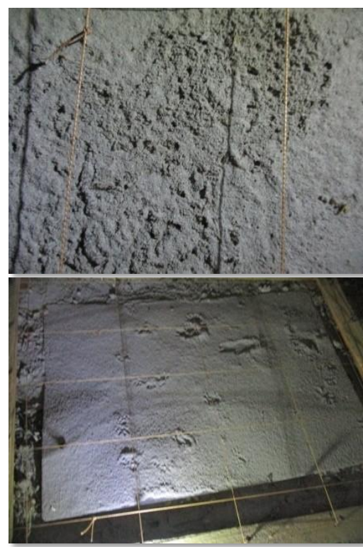
Examples of locally made rodent tracking tiles
