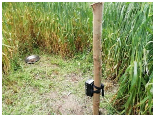
Infrared motion detector camera trap set in wheat field
