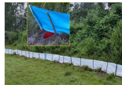
A bucket pitfall trapping line for rodent assessment
